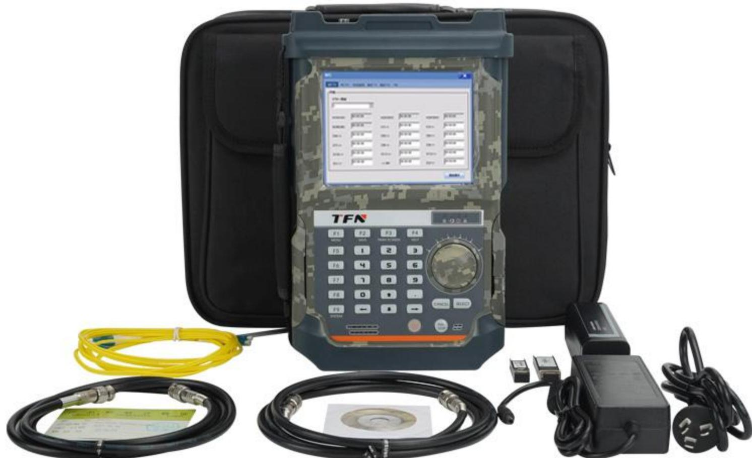
Host, instrument pack, battery, optical module, electronic CD, list, certificate of conformity, power adapter, 2M 75 ohm test cable LC/PC full duplex single-mode fiber optic test jumper, RJ48 to BNC test jumper
