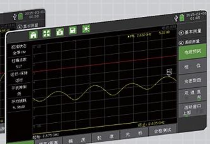
Figure 11 Cable loss test
