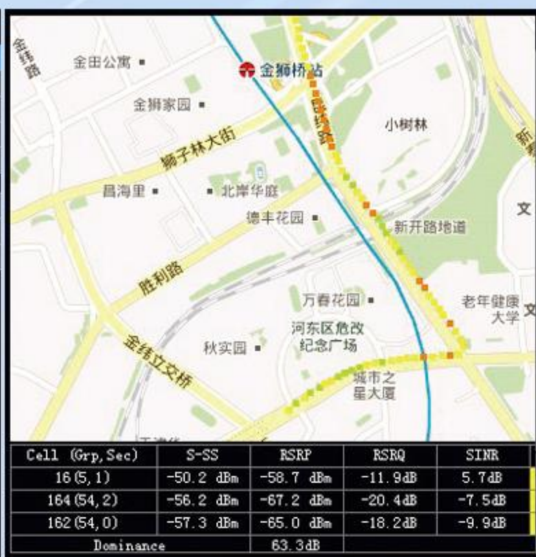
LTE coverage demodulation test
