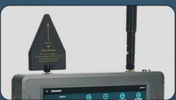
Support detection of commonly used communication frequency bands such as 315-433M, 800M, 1.2G1.4G, 2.4G, 5.2G, 5.8G, etc. Support external antennas to enhance detection and analysis accuracy
