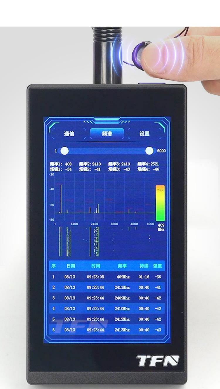
Spectrum function: If there is a suspicious device nearby, the field strength bar will change significantly and the signal strength of the suspicious device will be displayed at the bottom.
