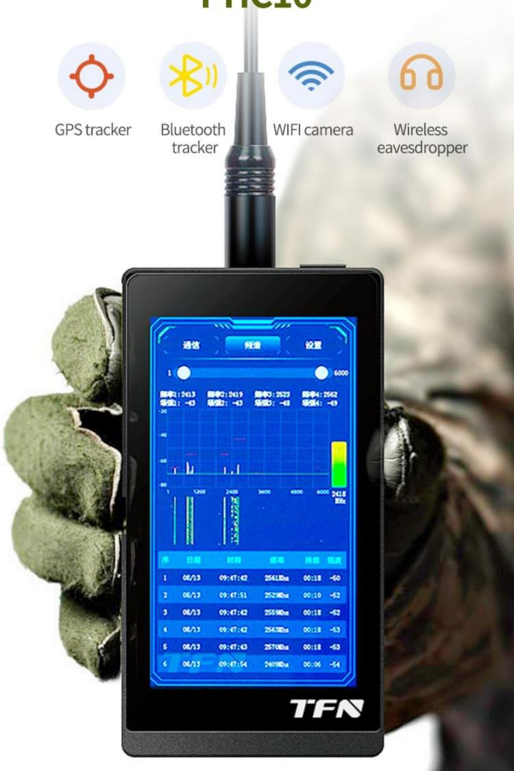
Detection of mobile phones, GPS trackers, GSM eavesdroppers, 3G/4G/5G video, Bluetooth and WIFI devices, storage and forwarding devices
